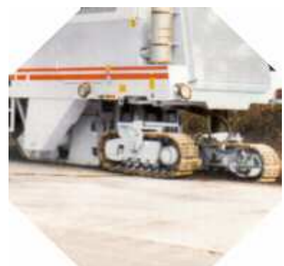
Wirtgen cold milling machine equipped with Felastec®-pad
