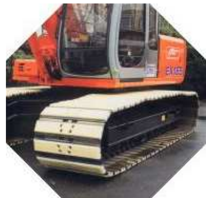
excavator fitted with Felastec® - pads
