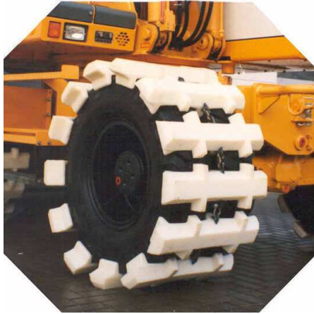
mobile-excavator equipped with Felastec® - anti-skid chains
